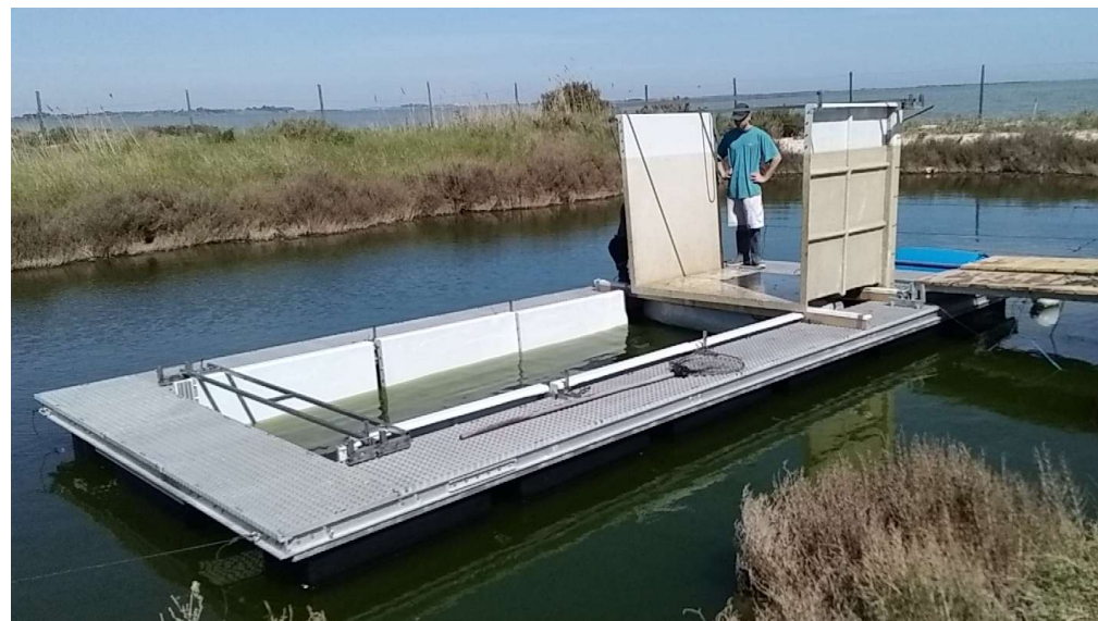
Assembly (bolting) of the 4 pieces (2,5 m 3 water per piece)
