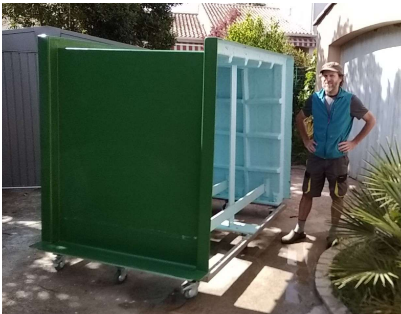
RFP mold for the pieces of the tank
